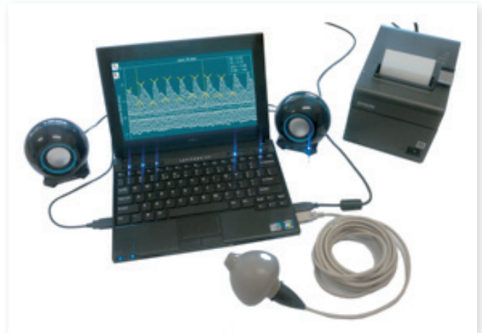
Figure 1 shows an example of the ultrasound probe plugged into a notebook via a USB-connector cable. Attached to the notebook is a thermal printer for result print-outs, and external speakers for audio amplification of signals.
